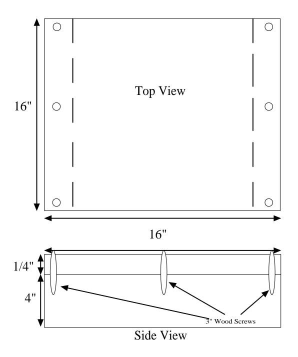
1 Each 16" X 16" Piece Of 1/4" Plywood Or Particle Board
